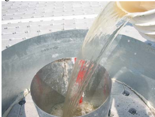
Figure 4. Surface inundation test.
