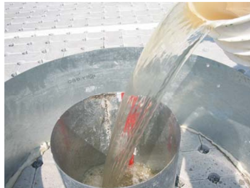
Figure 4. Surface inundation test.
