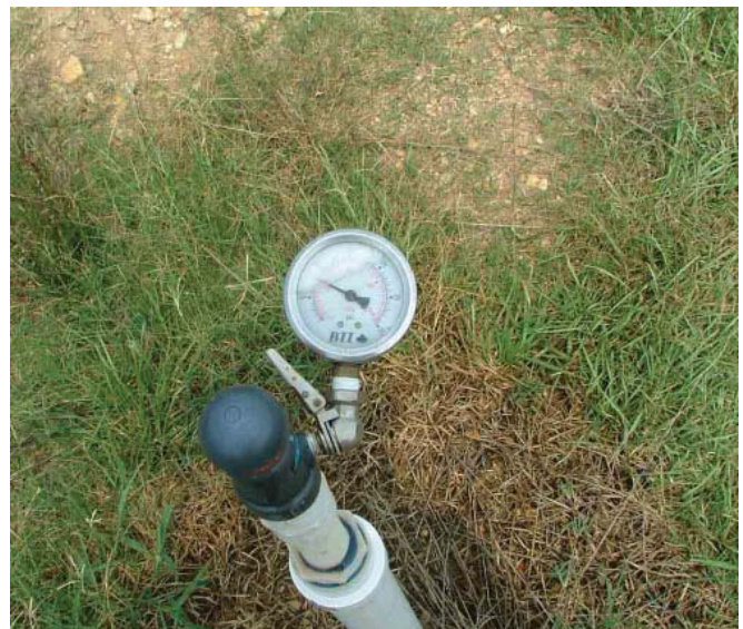
Figure 2. Monitoring pressure at several key locations is critical for SDI system evaluation.
