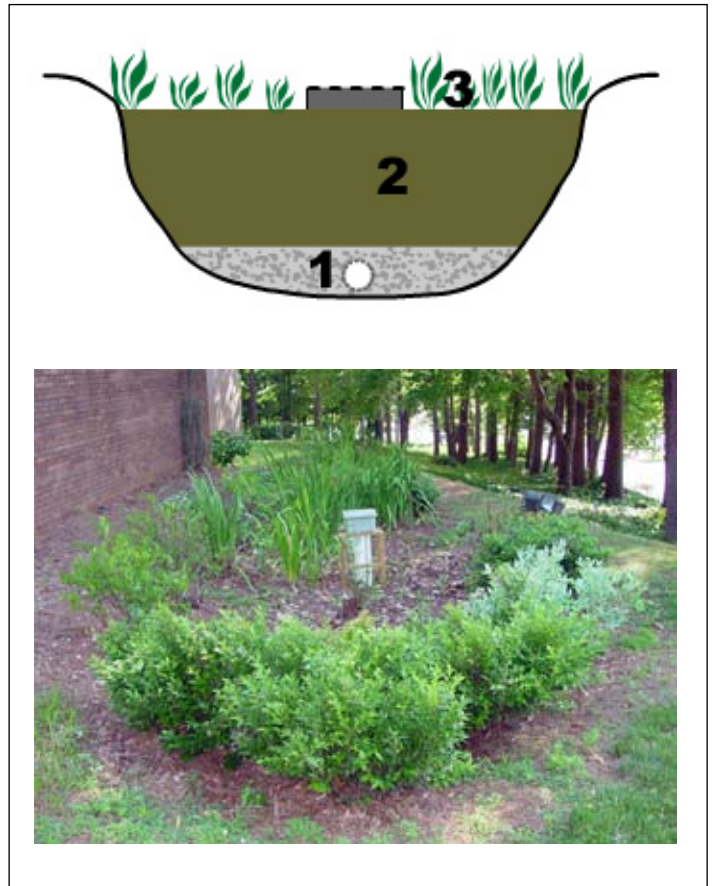
Figure 7. Cross-section of a typical bioretention area (top) and photo of an example (bottom)
