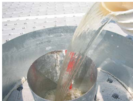
Figure 4. Surface inundation test.
