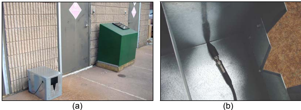
Figure 3. (a) Sampling equipment for WCC control roof. Weir box is on the left and green sampler storage box is on the right. (b) View inside the weir box with baffle, level sensor, and weir plate.
